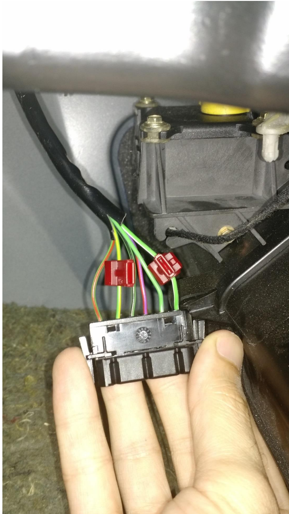
Figure 2b (Accelerator Pedal Position Sensor connections)
