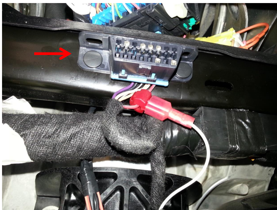
Figure 3 (OBD2 Power connection – General reference only not C5 specific)
