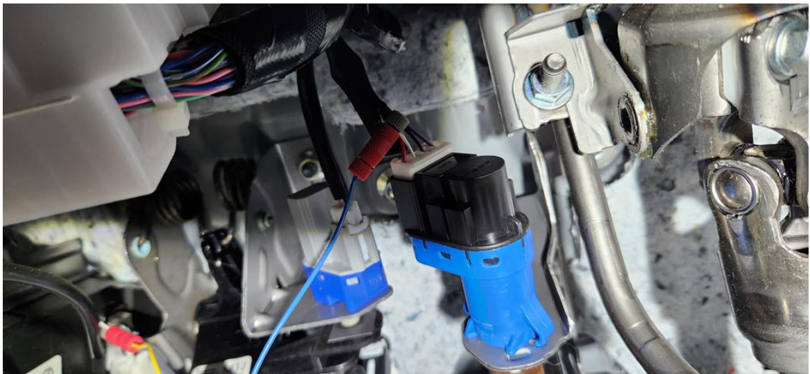
Figure 3B (Brake Sensor wire taps placement*) This picture is specific to Miata ND
