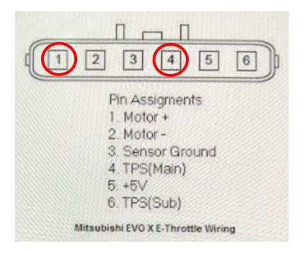
Connect Auto-Blip's Red wire and Green wire to EVO wires #1 and #4 (order does not matter)
