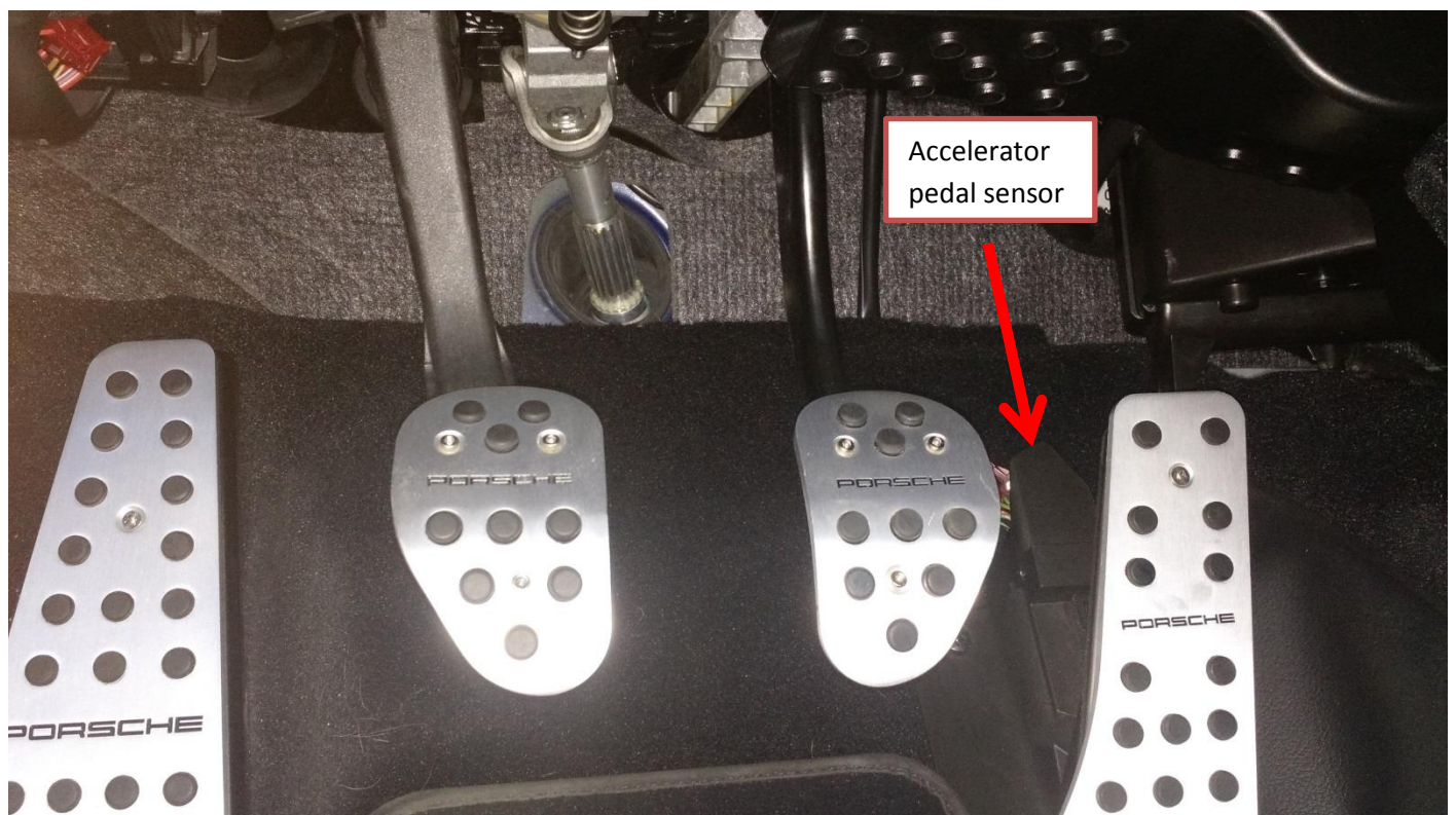
Figure 1b (General overview of the Sensors under the driver's dash)
