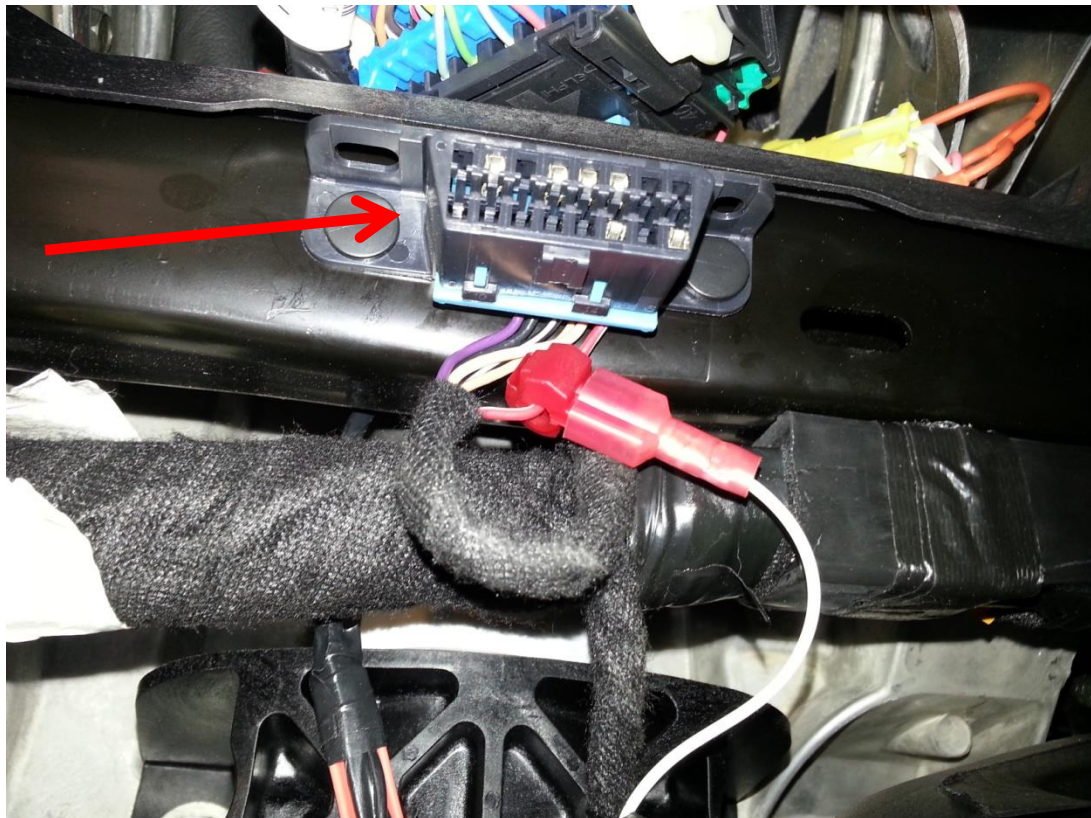
Figure 3 (OBDII Power connection)
