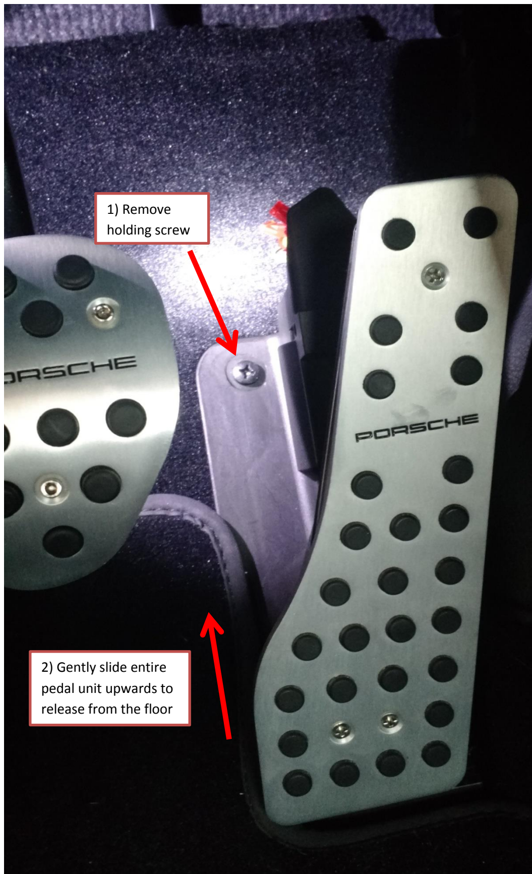
Figure 2a (Accelerator pedal removal recommended to access wire harness)
